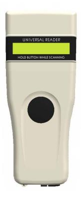
The Global Pocket Reader Plus (GPR Plus) is a portable hand-held PIT tag reader that provides cable-free operation and wireless communication via its integrated Bluetooth® module. The reader conforms to the technical specifications of ISO Standards 11784 and 11785 and reads all Biomark tags, FDX-B ISO, BioTherm13, HDX ISO, and FDX-A PIT tags.
